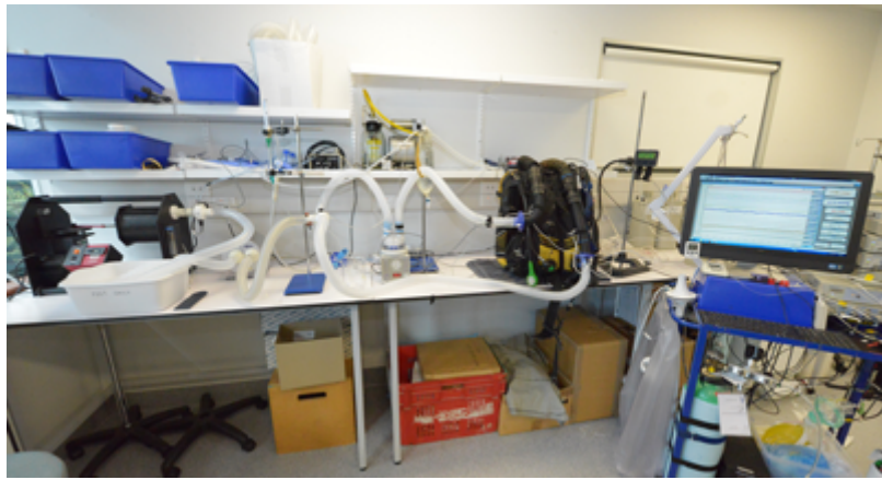
Figure 1 – Benchtop rebreather testing setup with an Inspiration Evo+ rebreather incorporated in a test circuit in which ventilation and CO 2 introduction simulated moderate exercise.
