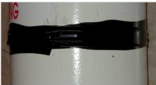
After you have affixed the electrical tape, install the hose clamp over it. Look at it from all sides to insure that it's not in direct contact with the bottle. Then put electrical tape over the hose clamp. As you can see, you'll need to run it over the nut twice to cover it completely.
