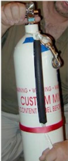
**Before tightening the hose clamp, make sure the rope is properly positioned.** The rope should run down the front of the bottle, directly below the valve opening.
